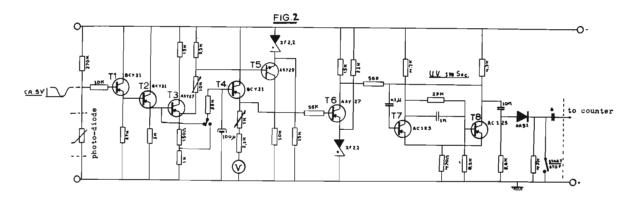
By means of this fly-counter a population of many thousands of flies can be counted within ten minutes with an error < 0.5%.
