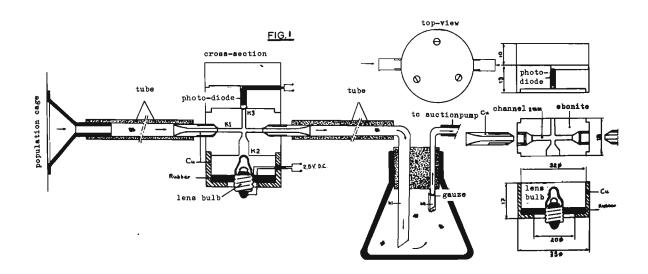
In the amplifier-discriminator and pulse-shaper, (fig. 2), the photodiode is connected in series with a resistance of 270 k  $\sigma$  connected to the -15 V. supply. The flies moving through  $k_1$  cause a negative impulse of about 5 V over the photodiode. The pulse width
